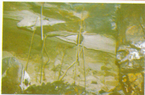
Cable bolted roof before and after blasting
