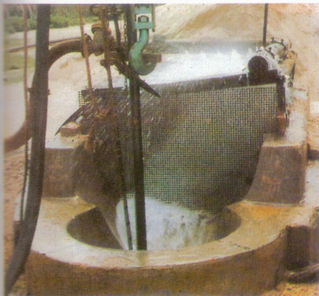
Sand / Water flushing arrangement
