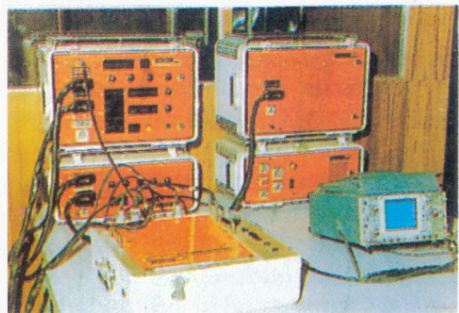
Digital seismic equipment for HRSS survey
